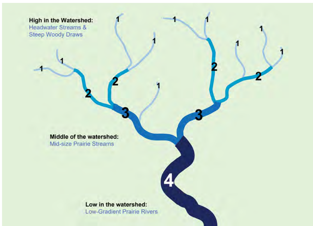
Figure 43: Stream order affects stream type. Streams labeled “1” are in the headwaters and are commonly referred to as first-order streams. They are dominated by overland flow of water and have no upstream concentrated flow. When two or more first-order streams merge, they form a second-order stream. Lower in the watershed, these second-order streams come together to form third-order streams, and so on. The larger the stream order number, the larger the area it drains. Graphic © Corissa Busse, TNC
