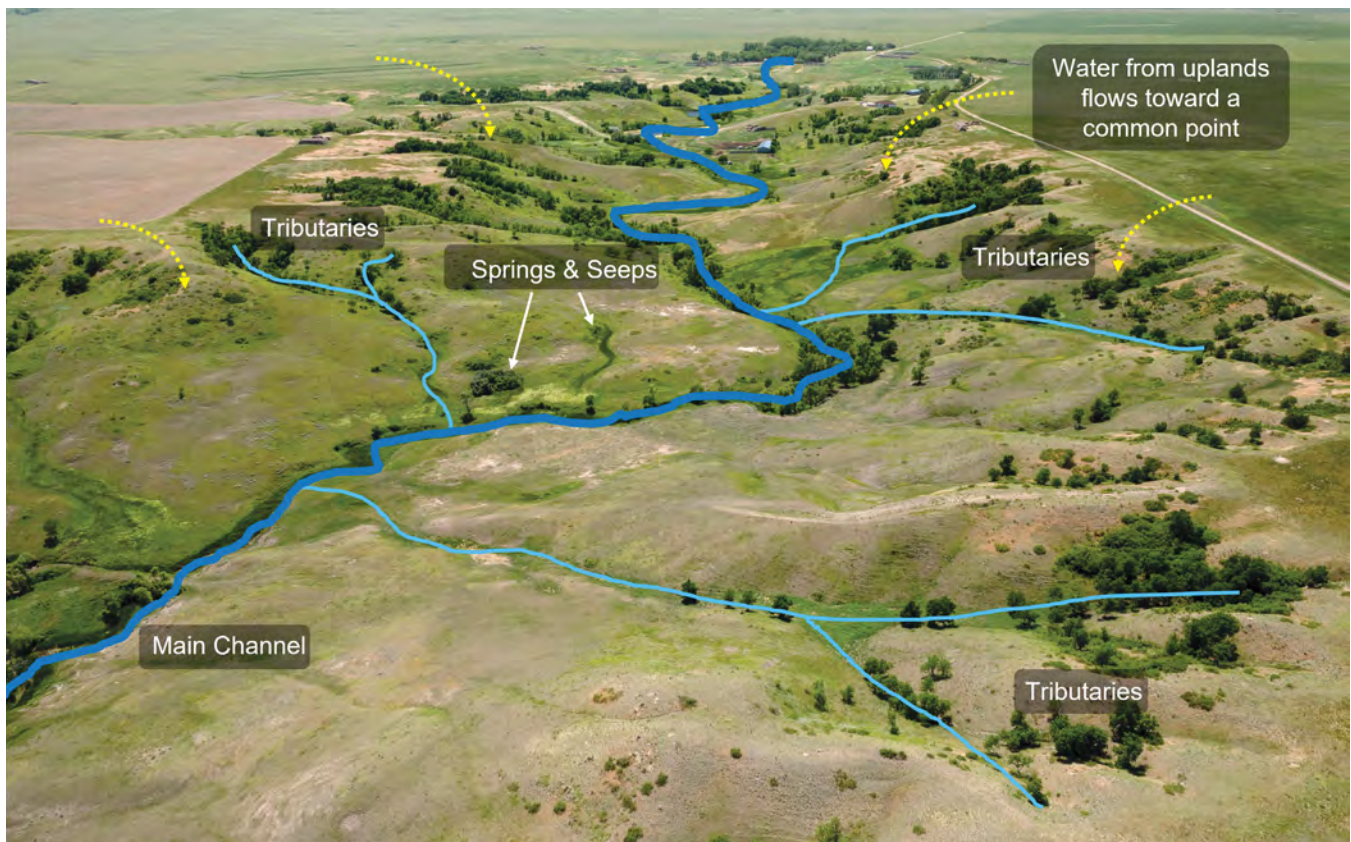
Figure 10: A watershed is an area of land that drains all the streams and rainfall to a common outlet such as a reservoir, or any point along a stream’s main channel. Watersheds can be small, such as in the picture here, or large, such as the entire Missouri River Basin. Photo © Joe Dickie, Generation Photography, Inc.
