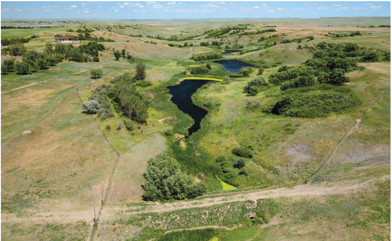
Figure 2. In the late 1940s, Clarence Mortenson installed a series of small check dams in Todd's draw to help slow and hold water, mimicking what beaver would have done. At the time, very few trees dotted this landscape which was very eroded.
