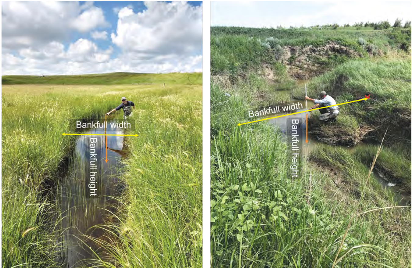
Figure 27: These images show the measuring of bankfull width and height (or the width of the channel and height of water when it just begins to fill the stream's banks before spilling into the floodplain). This measuring process is described more in the assessment portion of this guide. Photos © TNC
